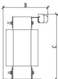
Side view of AITRseries isolation transformer
