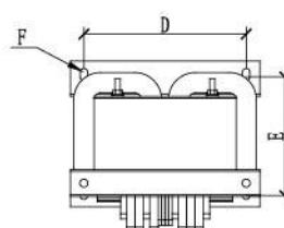
TOP view of AITRseries isolation transformer
